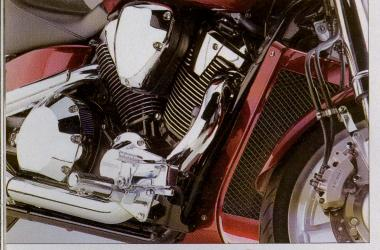
Our Spec 2 VTX came with a satin-black engine and milled cylinder-fin edges. Plainer Spec 1 has silver-painted motor, while Spec 3 uses more chromed and polished parts throughout, including an intense buff job on the five-spoke rims.
