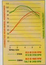
off idle was noticeably more crisp, and the torque increase from 2700 up to redline was significantly greater than stock. Indeed, at around 4100 rpm, the torque output was almost 9 ft.-lb. higher.
